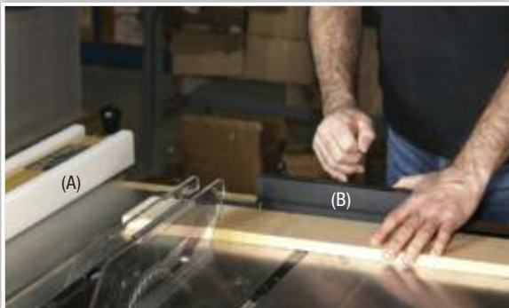
19. Never use fence(A) and the guide(B) at the same time. Do not force the blade into the cut. Use a feed rate that does not bog down the saw.
