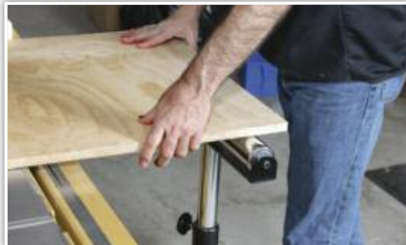
20. Use roller stands to support the large work-piece.
