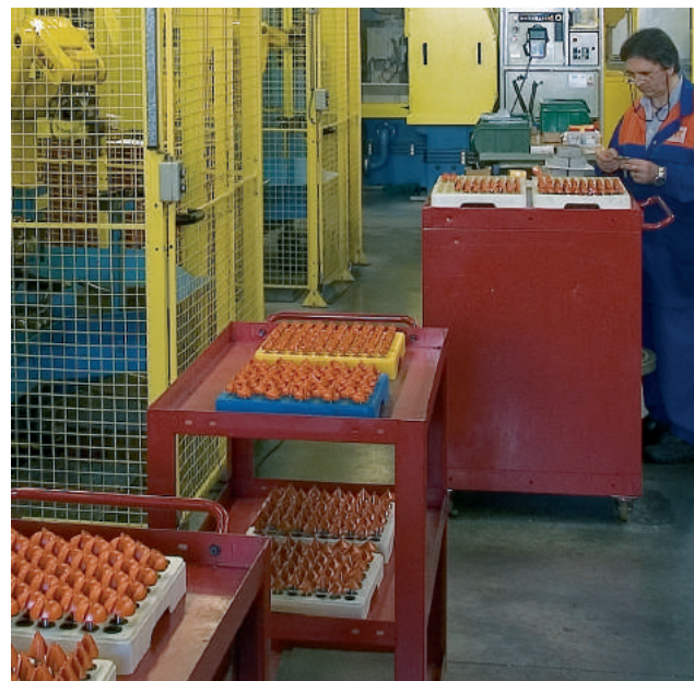
Loading the automated multi-axis CNC sharpening machines.
