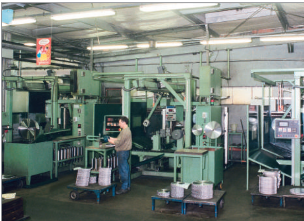
Grinding and tensioning the blades.
