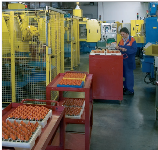
Loading the automated multi-axis CNC sharpening machines.
