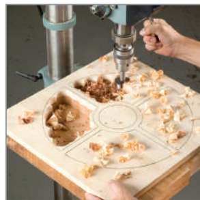
Rough out the interior using a drill press and a 2" Forstner bit.
