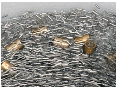
Stainless steel pin media reaches burrs other media can't touch.
