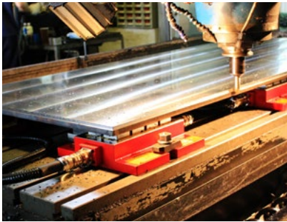
Use for fast setups on plate stock
