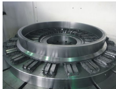
Even workholding - no part distortion
