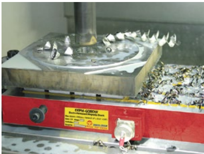
High holding power for heavy cutting
