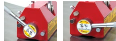
Lever in the "ON" position engages safety lock.
