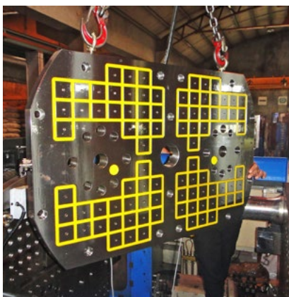
Load and install PIM magnet with bolts
