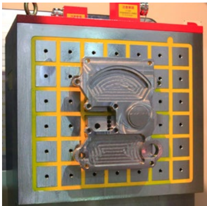
Complex part shapes - 5 sides machining
