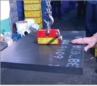
3.5 X Safety Factor above rated load capacity
