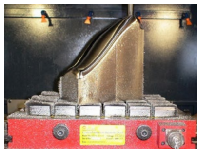
Slope milling unusual parts or 5-axis
