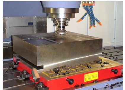
Face milling on workpiece with work-stops installed
