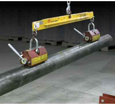
Use spreader bars for long, difficult round stock
