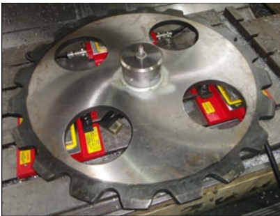
Large tooth sprocket being machined
