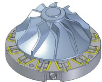
5-axis turbine blade machining
