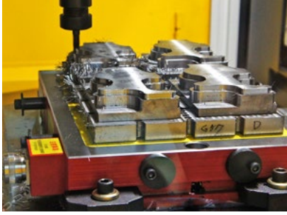
Gang part setups together and still machine
