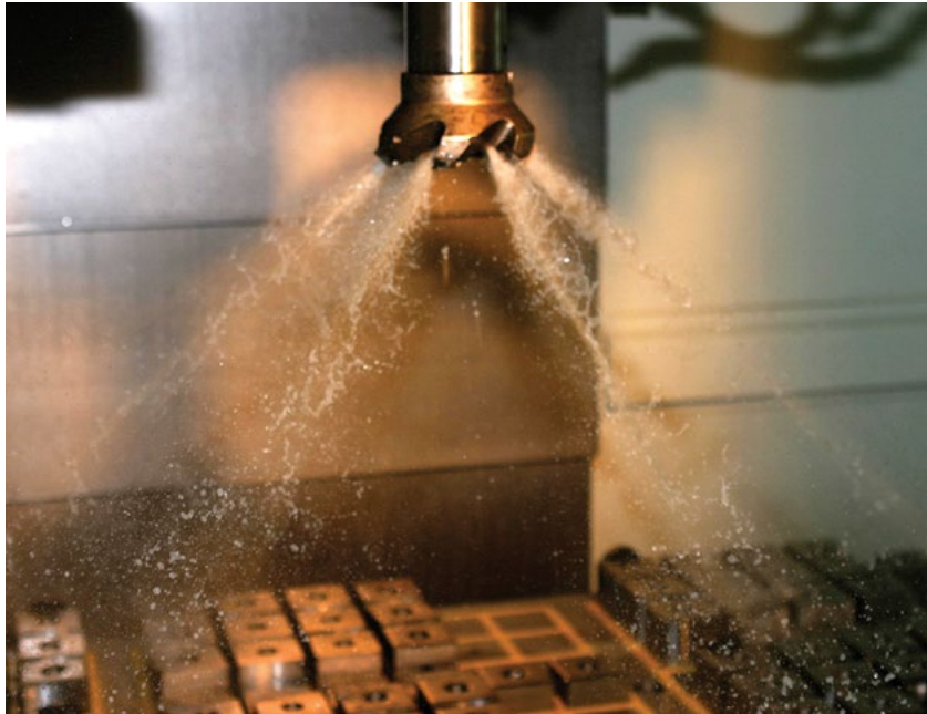
CoolBLAST arbor screw provides coolant path.
