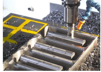
Machining mold cavities
