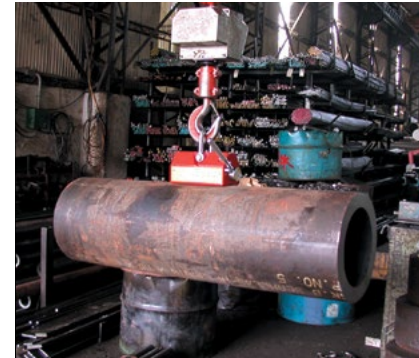
Beveled bottom surface lifts round stock.
