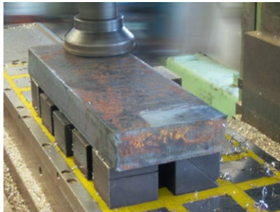
Use spring-loaded blocks for warped stock
