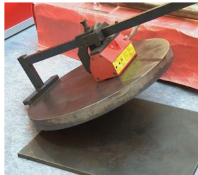
Move round or rectangular stock vertically.
