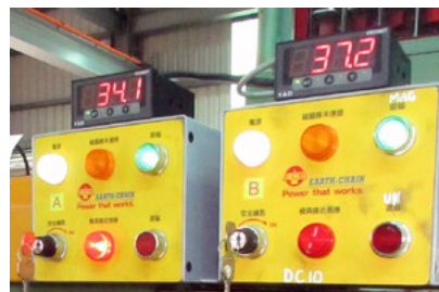
Controls require operator to use both hands.
