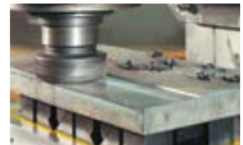
Milling warped stock with induction blocks
